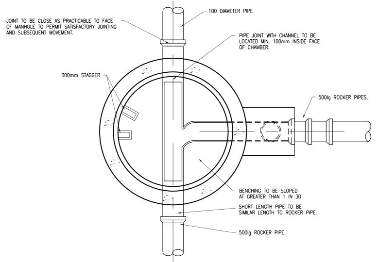
BACKDROP MANHOLE DEPTH TO SOFFIT 1.35 TO 3.0m
